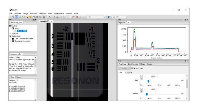
The image below shows a scan with laser drift, meaning the plot of the cross section appears with lines that are not flat. Notice how the intensity varies across the cross section, but compared to the dirty tile, it has a smooth profile. Typically, recalibrating the scan can remove this type of variation. If recalibration does not work, try to clean or realign your calibration material.
